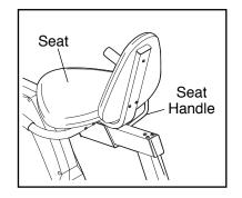
adjust the seat, make sure that your knees will not touch the handlebar or the console when you pedal. To adjust the seat, first pivot the seat handle to
